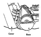
Tilt cover to back. Press cover firmly until side tabs snap into place. Replace cover screws, light bulb and light cover.
