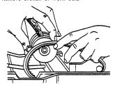
Slide brush supports off to check and clean brush support areas. See Brush Assembly for picture of complete brush.
