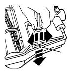
Turn brush over. To remove cover, insert screwdriver at cover tabs on both sides and twist to release tabs.
