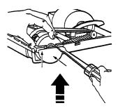
6) Remove broken or worn belt.
