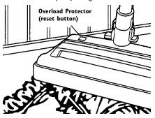
Press reset button on top of the brush. Plug in and turn on vacuum and brush.
